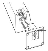
3 Reattach the speaker stand by engaging the protrusions on the stand in the holes for either a vertical or upward angle.
